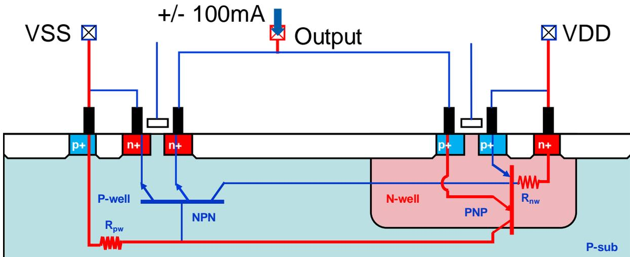
Figure 2: Cross-section of Parasitic Thyristor in CMOS Buffer
