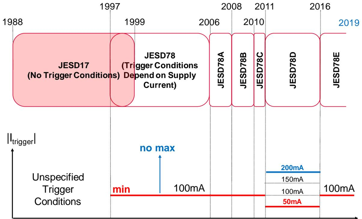
Figure 1: Latch-up Testing Method Revisions and Associated Current Injection Requirements
