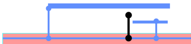
Figure C2d: Create an additional mechanical “ESD trap” to guide ESD for an alternative route.
