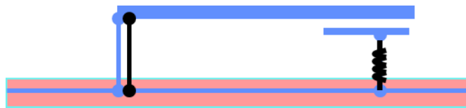
Figure C2c: Better grounding, while increasing the impedance of the small board grounding. Note that this solution makes the small board more sensitive to other RF noises.
